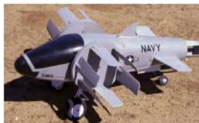
Figure 2.14: Bosch Aerospace cycloidal propulsion system [8]
